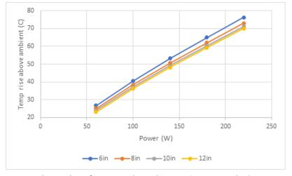
\*Thermal Performance based on a 40mm LED device.
